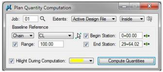
**NOTE:** To limit the extent of calculation set Extents: to Station Range, and set the limits desired in the *Baseline Reference* portion of the dialog.
